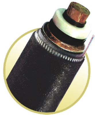
Model: ZS-YJQ41 + OFC Single core (copper) XLPE insulation, Lead sheath, Steel wire armor, Yarn serving submarine cable
